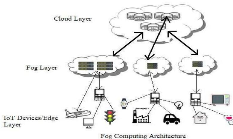
Figure 1. Fog Computing Structural Design
