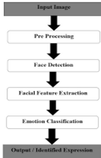
**Figure. 1** Basic Process of Face Recognition
