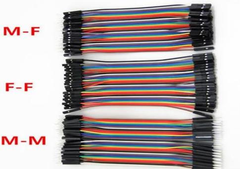
Fig.10 Jumper Wires
