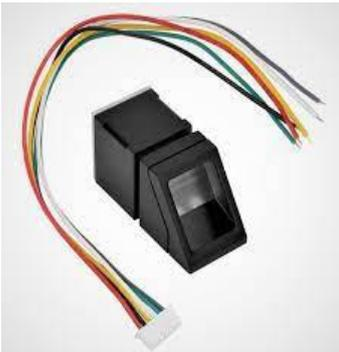
Fig. 4 R307 Fingerprint Sensor
