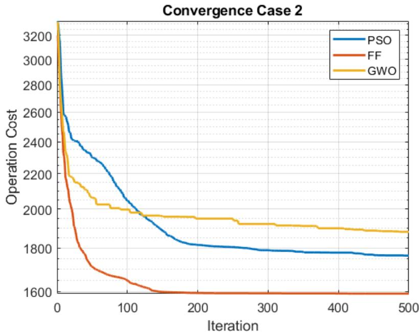
Figure 9: Scenario 2 convergence characteristic of firefly algorithm compare with other techniques
