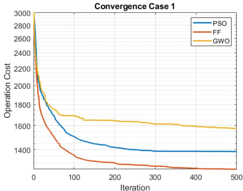
Figure 4: Scenario 1 convergence characteristic of firefly algorithm compare with other techniques
