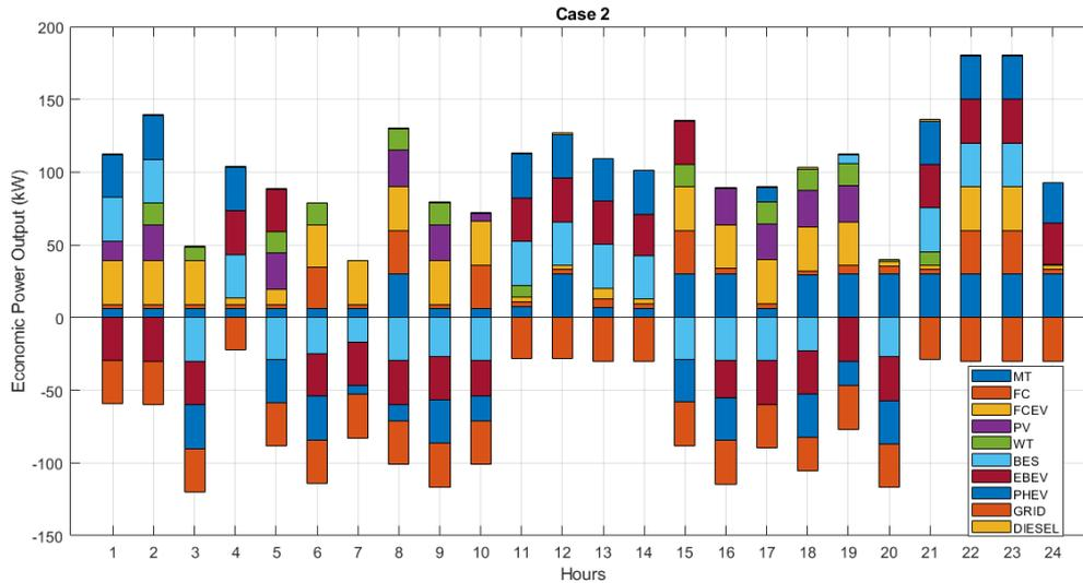
Figure 8: Scenario 2 Output of the various microgrid components using fire fly algorithm for 24 hour operation duration
