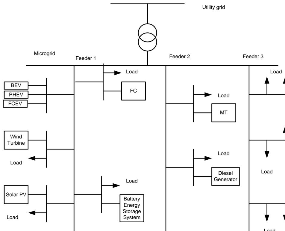
**Figure 2:** Proposed grid-connected microgrid configuration
